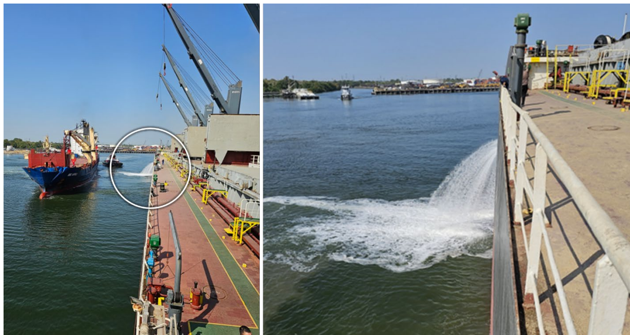
Figure 5. Left to right: BBC Africa (left) and Common Faith after the collision. Common Faith punctured port ballast tank spilling ballast water (circled; left photo). (Source: Common Faith master)
