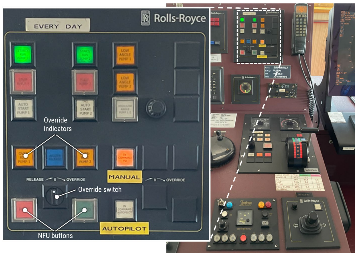
Figure 3. BBC Africa main bridge control station. Inset shows the emergency override portion of the steering panel with its NFU buttons, override switch, and override indication lights labeled.
